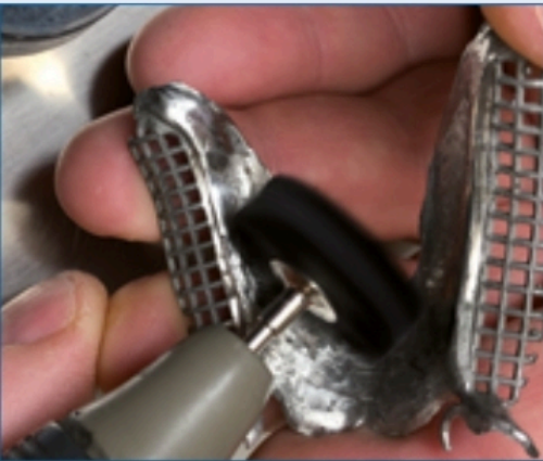
MiniVliesBürste - schwarz / Chunking + Vlieseinlage MiniScotchBriteBrush - black / Chungking with scotch brite insert
