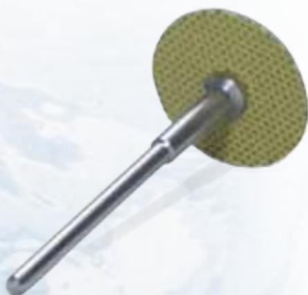
Textile carrier material with one-sided diamond coating (during use place the diamond-coated side towards the shank). High flexibility of the discs enables a perfect adaptation to workpieces.
